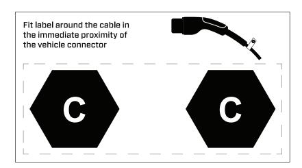
2. Fit label around the cable in the immediate proximity of the vehicle connector.
